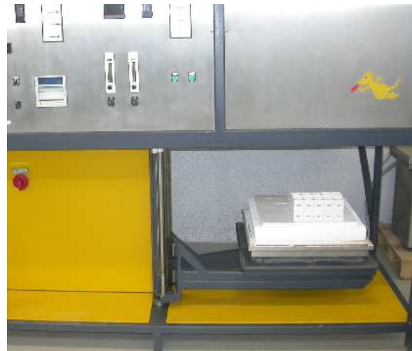
Fig. 5: Chamber-kiln with sintertrays
