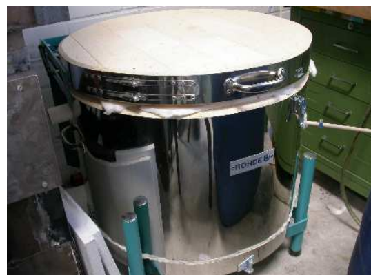
Fig. 4: Top loading kiln with connection to nitrogen gas flow
