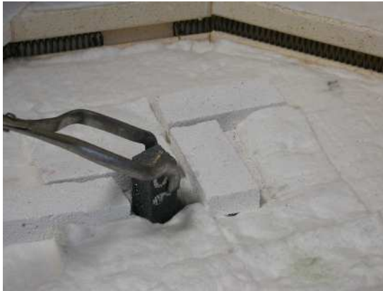
Fig. 5: Charging of specimen through the multi layer kiln sealing
