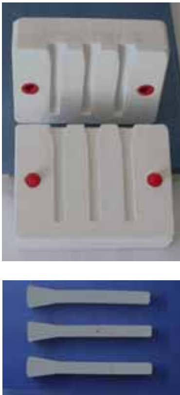
Fig. 2 Casting of samples top: plaster mould, bottom: cast samples
